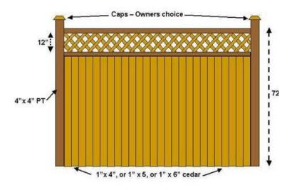
The fence design adopted and approved by the Board is shown here. It is 72" tall, constructed from 1 x 4 cedar with a 12" cedar lattice strip across the top. Support posts need not be cedar, but can be pressure treated lumber. Approved finishes
